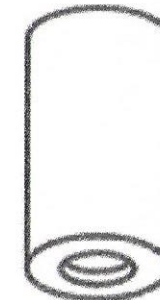
#21 Install cup O.D.: 2" I.O.: 1-3/4" Length: 3"
