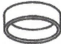
#07 Receiving tube O.D.: 2-1/2" I.O.: 2-1/4" Length: 3/4"
