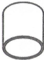
#17 Receiving tube O.D.: 2-1/2" I.O.: 2-1/4" Length: 2-3/4"
