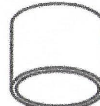
#14 Receiving tube O.D.: 2-3/4" I.O.: 1-7/16" Length: 2-1/4"
