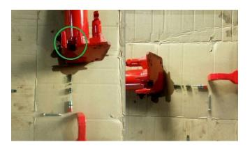
If the unit sits unused for a week or more at a time; you may need to remove and reinstall the return valve to ensure smooth operation.
