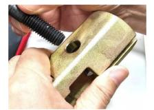
After fitting the incjetor, insert the screw bolt to the hole on plate B (without thread).
